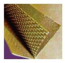
High-Temperature Gasket Material based on Mica with Perforated Stainless Steel Reinforcement 1.4401(AISI 316). It is specifically designed for hot, dry gas applications up to 900°C and 5 bar. However, the outstanding chemicals resistance of mica makes the gasket suitable for a wide range of other applications. Also available as Milam H ,high quality homogeneous mica sheet.
